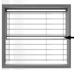
Left: Example of multiple guards stacked in single/double hung window. Open space between guards should not exceed 4 inches.
