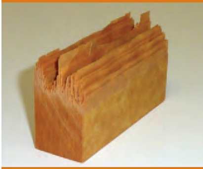
A cross-section of Richlite shows how this countertop material is made up of layers of recycled paper.
